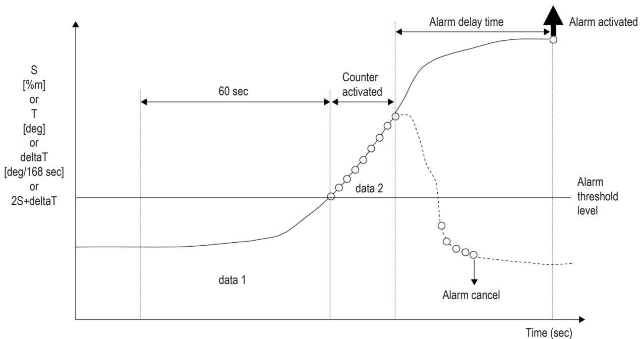
**Maximum alarm delay time is 60 seconds.**
