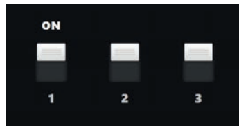
Setting for Exit light (All switches ON)
