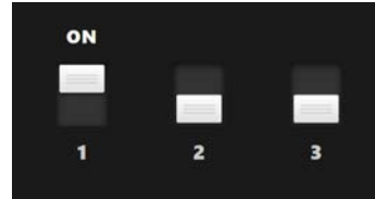
Setting for Emergency light (Switch 1 ON)
