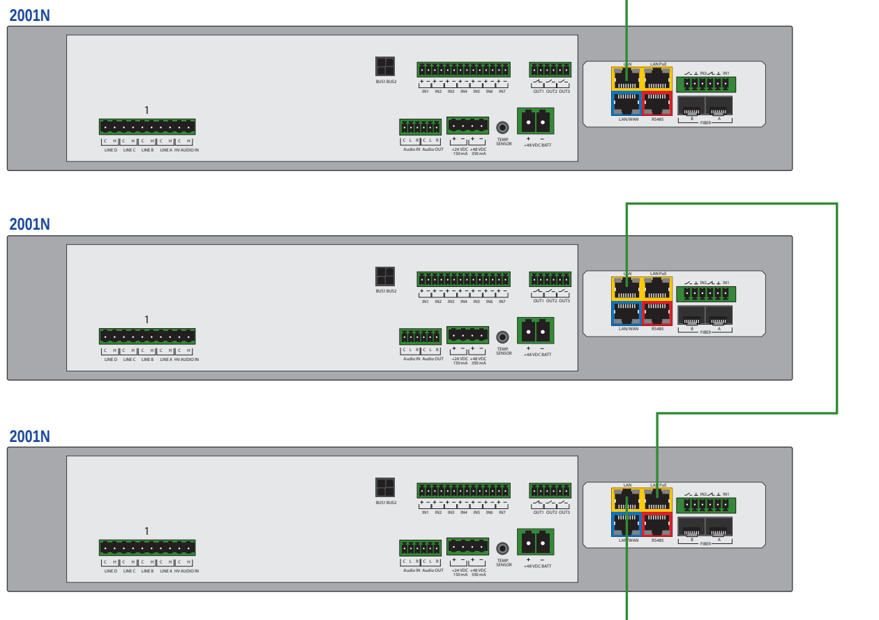
Drawing 45. Example of CHAIN topology control units connection
